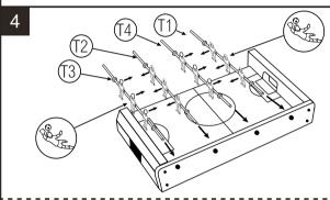
Install the 4x Player Rod (#T1, #T2, #T3, #T4) into the pre-drilled holes along the side of the Side Panel (#E2).
