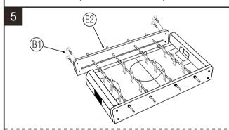
Position the remaining Side Panel (#E2) and attach securely as in step 1 using 4x Bolt (#B1).
