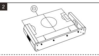
Insert the Playing Field (#E3) into grooves of the assembled pieces from step 1 as shown.
