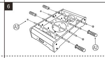
Attach 4x Handle (#A2) and 4x End Cap (#A3) as shown and press firmly into place.
