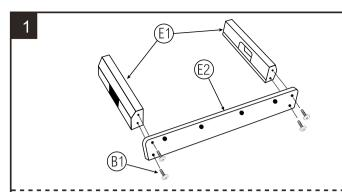
Use 4x Bolt (#B1) to attach 2x Goal End Panel (#E1) and 1x Side Panel (#E2) with Tool provided.
