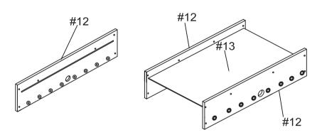
Put #12 Side Panels x 2 pcs and #13 Playing Field up-side down, insert the #13 Playing Field into the groove on inside of #12 Side Panel.
