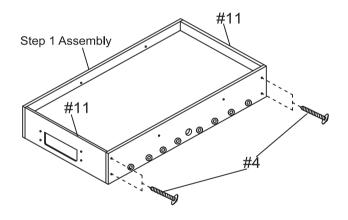
Attach #11 End Panels x 2 pcs to Step-1 Assembly using #4 Screw x 2 pcs for each end to fix them together Repeat for all 4 ends.
