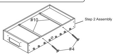
Attach #10 Playfield Support Brace to Step-2 assembly by using #4 Screw x 2 pcs.
