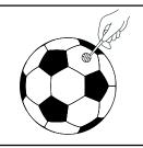
STEP 9: Use the tool if necessary to adjust the cap securely into place.
